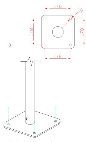
Fix Surface Plate to the ground surface **Ground Anchors Not provided**cover fixings with caps provided
