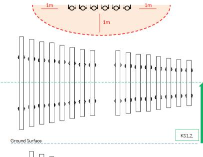
Install Instrument with 1m free space (from widest point) around t.
