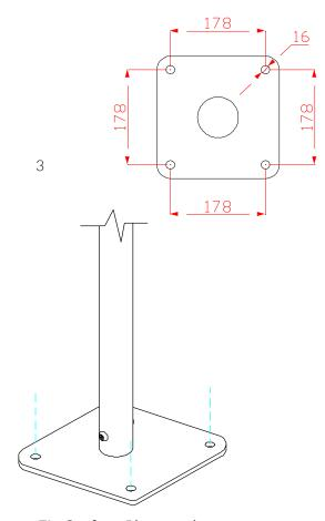
Fix Surface Plate to the ground surface **Ground Anchors Not provided**cover fixings with caps provided
