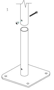
Locate the Surface fix Plate into the leg of the instrument.
