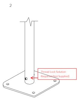
Fix instrument to Surface fix plate using M10 bolt and Barrel Nut and use **thread locking solution** to prevent fixings working loose.
